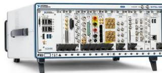
Figure 1.6 *PXI Instrumentation Platform (ATE)*
